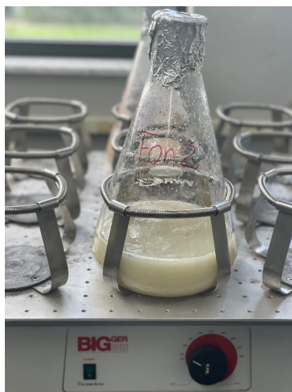
Figure 3. Flask of inoculum in liquid culture on a rotary shaker at 25°C (Sakata)
