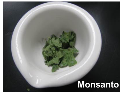
Fig. 6. Frozen fresh symptomatic tissue to be homogenized with a mortar and pestle in cold buffer
